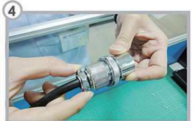
4 半月邊壓入（與線材不能留有間隙） Crescent-shaped clamp mounted (The gap couldn't be allowed with the cable connected)
