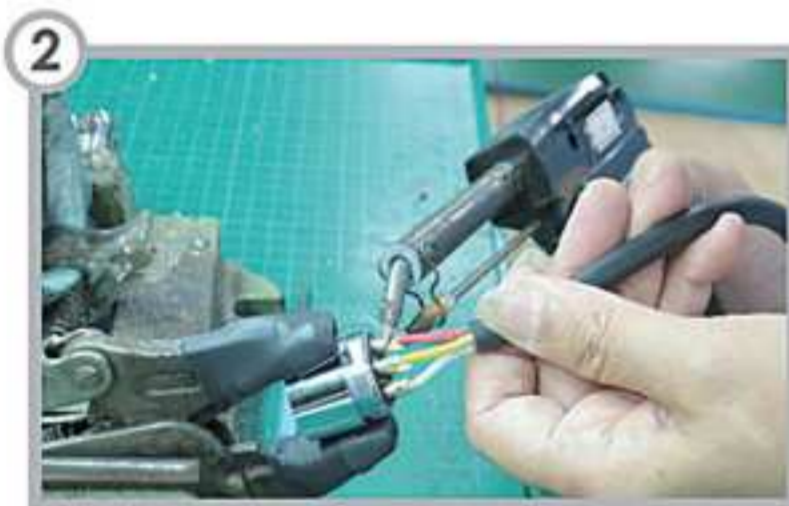
2 使用夾具將接頭夾持住，線材裸線與上固定體的接觸體缺口進行焊線加工 Using the clamp to fix the connector Doing soldering assembly between the bar wire and upper body
