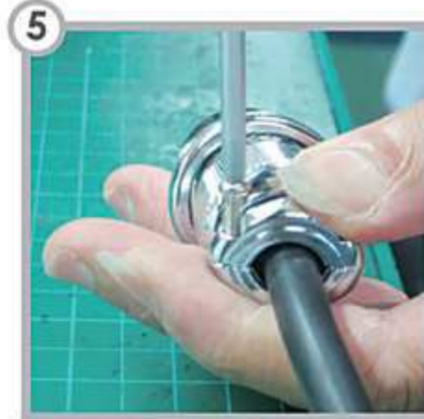
5 固定螺絲（圓頭十字 x 2支）鎖緊 With 2 screws (Round head) screwed tight
